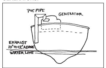
Determine how large a generator you will need. Don't underestimate the wattage, as your lights will be dim. Rentals are available, pay in advance if necessary to reserve yours. Mount the Generator securely on an open deck area where an exhaust extender hose can go over the side away from decorations. The generator can be placed on a piece of carpet and held down with 2x4s to help deaden the noise.
